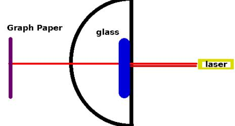
Getting the beam centered on one of the dark lines is surprisingly hard. I may consider cutting a slit on the graph paper on one of the darker lines so that light will pass through. So if you see a cut on the graph
