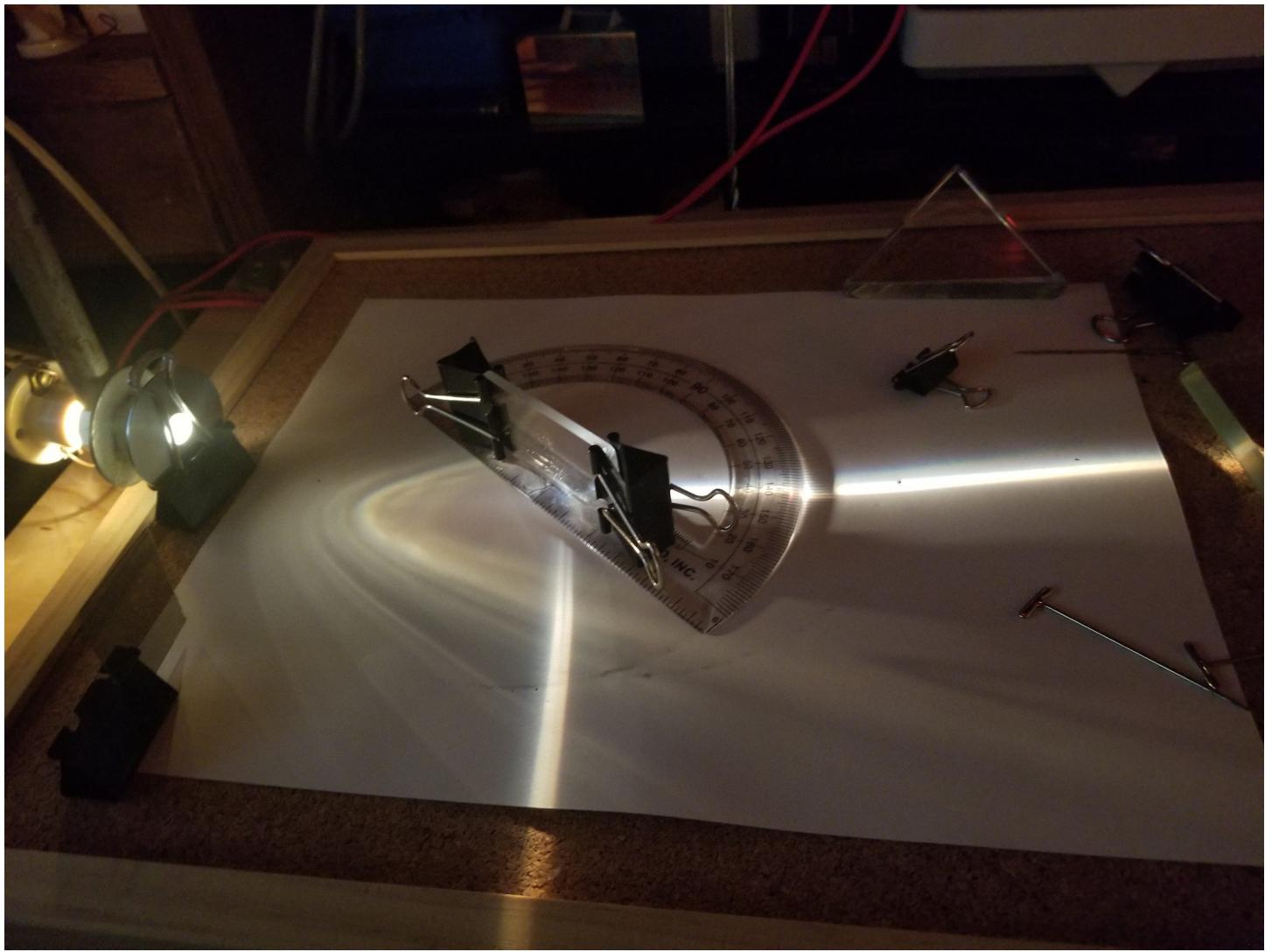
This shows transmission and reflection beams. In fact, this is also close to Brewster's angle. Notice that the beam you see on the paper from transmission and the reflected beam are not at 90 degrees because it is only inside the glass that the transmission beam is at an angle of 90 degrees with the reflected beam. Seeing the beam inside the glass is not easy. However measurement of polarization is doable.
