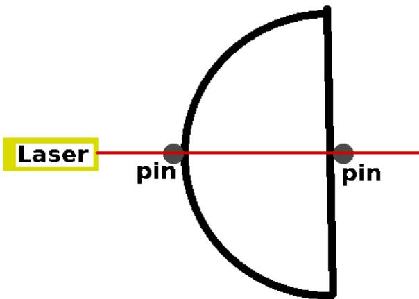
You will need to optically align your system. The image to the left shows how to do this. Align your system first by putting a pin behind the nail in the protractor and place a second pin in front of the protractor at 90 degrees. Then align your system so that the laser light hits both pins.
