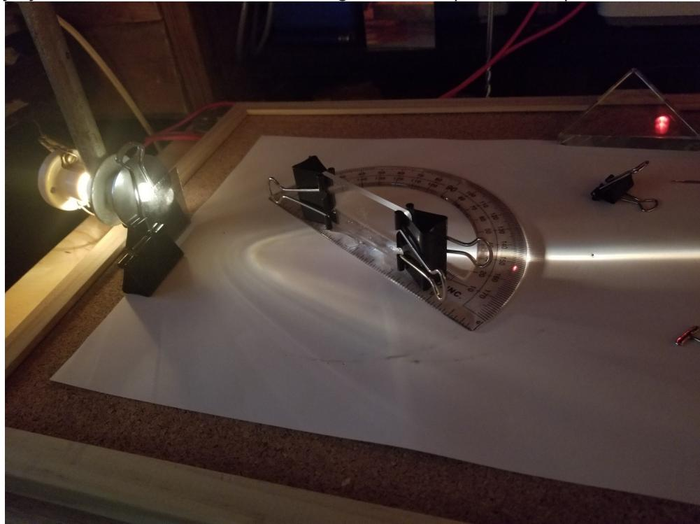
My system at Brewster's Angle. Notice the second surface reflection is not extinguished with the polarizer. However the first surface reflection is.
