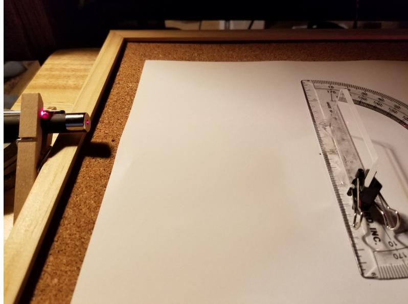
My glass slab. Your slab will have clamps on each side. Note the reflected dot is directed back into the laser.
