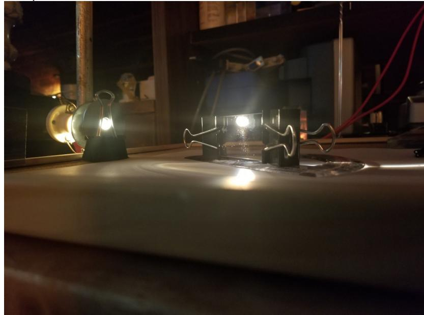
To orient your polizer, rotate the polarizer until the beam is at it's dimmest. The holder clamp for the polarizer should be such that it will hold the polarizer in the orientation when placed in front of the incoming beam.
