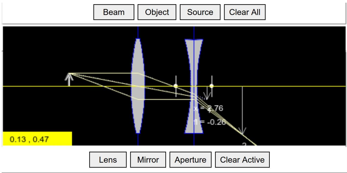
So long as you do not move the lens so far from the virtual object so that it is outside the focal length of the diverging lens, an image will form. In practice we won't have a problem with that in lab since our meter stick is only  $1$  m long.
