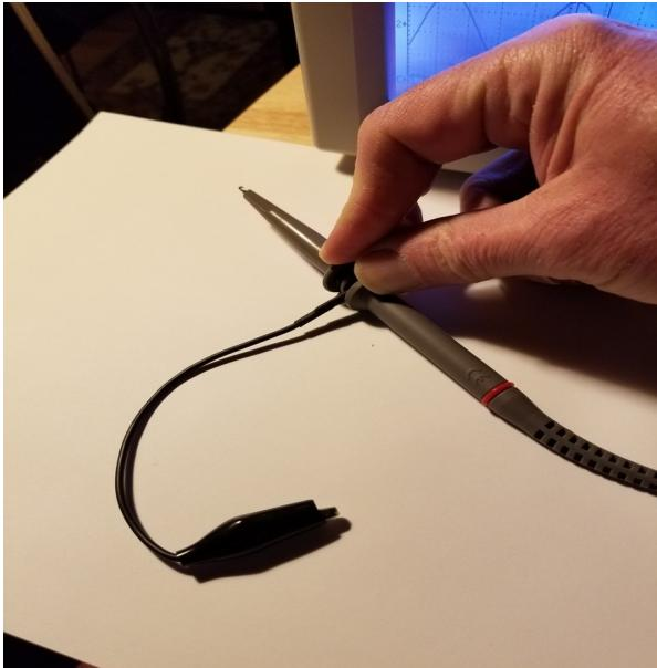
In this image to the left, the red band is visible. The black clip is the ground connection and the probe connector can be seen by pulling back on the probe head as I have indicated in the image. Also, less visible but on the side of these probes is a switch for 1x and 10x. This is a reference to the internal calibrated resistance of the probe. Your probe should be set to 1x only.
