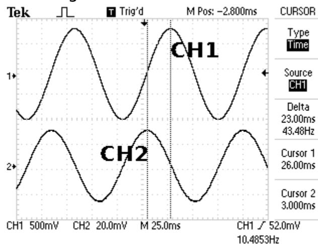
The image above shows the correct cursor settings that will allow a measurement of the time between those two peaks. By knowing the frequency (which the scope will measure) you can then determine the phase. Note that at resonance, the two peaks will have zero phase and at high frequencies, Ch2 will shift towards a positive phase shift. Below is a screen dump at 1000 Hz.
