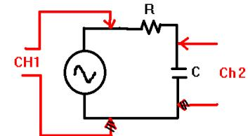
In the limits of low frequency  $A_v$  is 1 and for high frequencies,  $A_v$  approaches zero.
