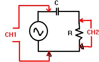
In the limits of low frequency  $A_v$  is zero and for high frequencies,  $A_v$  approaches 1.
