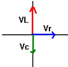
We can write this in terms of two vectors now using the difference between  $V_L$  and  $V_C$ .
