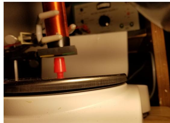
Now you need (before making measurements) to apply current and insure that a **positive current results in a negative scale reading**. It is best to tare the system at zero current before this. If you get a positive current with a positive scale reading, you will need to reverse the directions of the magnet in the cap.
