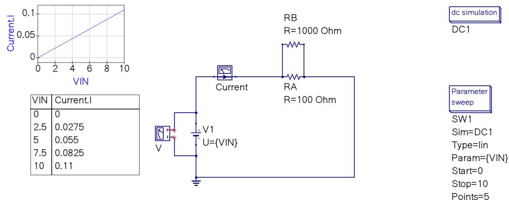
If you run the simulation under qucs, you might want to delete the voltmeter since it is already measured. It also gives a less than important error.
