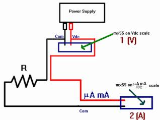
Here, we will use a variable voltage supply to vary the applied voltage to a resistance. You need to be a bit careful when making connections with analog meters (such as the voltmeters we are using) since you need to observe polarity. Basically, you want to connect red terminals to each other and black terminals to black terminals. The conventional current goes from red to black. The physical current goes from black to red.
