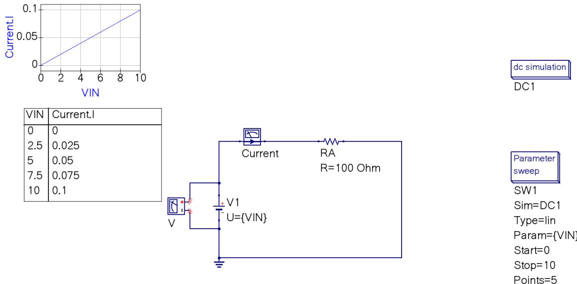
If you run the simulation under qucs, you might want to delete the voltmeter since it is already measured. It also gives a less than important error.
