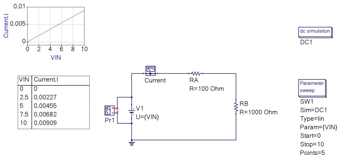
If you run the simulation under qucs, you might want to delete the voltmeter since it is already measured. It also gives a less than important error.
