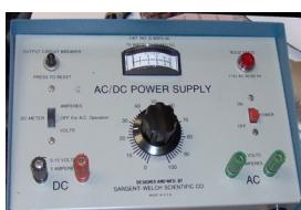
For DC operation, the black switch should be set to Volts or Amperes. This refers to the reading that is present on the meter above the word "Power". Use the black and red terminals for DC operation and green terminals for AC operation. We use black and red today.
