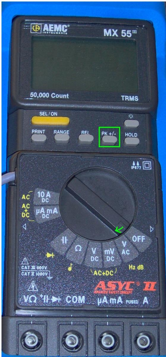
In order to initialize the mx55 serial interface, **the button pk+/- must be held while switching the meter on**. I have drawn a bright green box around the important button. If your meter is properly initialized to use the RS232 interface, it should show a small double-headed arrow in the display that says RS232.
