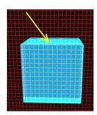
(1) Suppose for monochromatic light, the index of refraction of a slab is n and the glass slab has a thickness t. Find the displacement d of the light after it passes through the slab from the undeviated path of the light. Assume the cube is surrounded by air.
