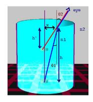
Seen from above the water surface, the coin appears to be at the intersection of the ray entering the eye and the vertical passing through the coin. Applying Snell's law to the water-air surface gives,
