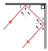
Solution: Consider the retroreflector construction shown. It consists of two mirrors placed at 90 degrees to each other.
