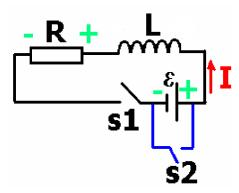
(1) Time dependence of a RL circuit. You know that Faraday's law says  $\mathcal{E}=-L\frac{\Delta I}{\Delta t}$ . Suppose you have a series RL circuit as shown. At t=0, leave s2 open but close s1. The question is how does the current through the circuit behave with time?
