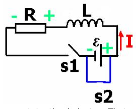
(2) Suppose that at some long time after s1 is closed, you obtain the theoretical maximum current through the circuit  $I=\frac{\mathcal{E}}{R}$  .Now, leaving s1 closed, close switch s2. Describe the time dependence of the current through the circuit.
