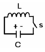
(3) Consider the circuit shown. Initially the capacitor has a charge Q. At t=0, the switch s is closed. Describe the time dependence of the circuit.
