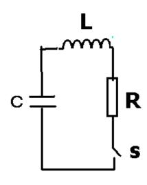
(4) The RLC circuit. Suppose that at t=0, the capacitor has a total charge  $Q_0$ . Then, the switch is closed. Describe the subsequent behavior of the circuit.
