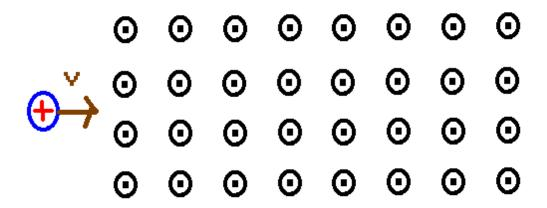
A charged particle moving at right angles to a magnetic field will be deviated by an apparent force which acts at right angles to the instantaneous velocity.
