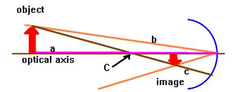
II: How does ray tracing lead to the mirror equation?
