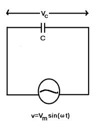
This analysis is valid if the circuit contains only a capacitor and the applied voltage must vary as:
