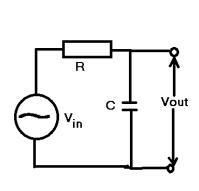
$$A_{v} = \frac{V_{out}}{V_{in}} = \frac{I_{m}X_{c}}{I_{m}Z} = \frac{\left(\frac{1}{\omega C}\right)}{\sqrt{R^{2} + \left(\frac{1}{\omega C}\right)^{2}}} = \frac{1}{\sqrt{(\omega RC)^{2} + 1}}$$
