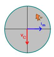
The current reaches its peak value 1/4 of a cycle sooner than the voltage reaches its peak value. For this reason, in this type of circuit obeying the initial assumptions it is said that the *current* always leads the voltage across a capacitor by 90°
