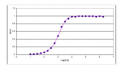
Notice that the HF response is that which would happen for the capacitor if it were replaced by a piece of wire.
