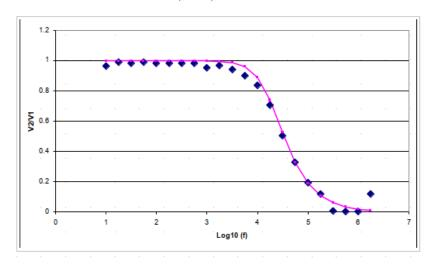
Note that at high frequencies, this acts much like a short across the capacitor. Now a question for you: suppose you replace the capacitor in these two circuits with an inductor. What are the response functions in those cases?
