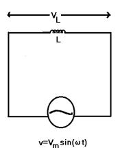
This analysis is valid if the circuit contains only an inductor and the applied voltage must vary as:
