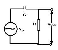
$$A_{v} = \frac{V_{out}}{V_{in}} = \frac{I_{m}R}{I_{m}Z} = \frac{R}{\sqrt{R^{2} + X_{C}^{2}}} = \frac{R}{\sqrt{R^{2} + \left(\frac{1}{\omega C}\right)^{2}}} = \frac{\omega RC}{\sqrt{(\omega RC)^{2} + 1}}$$
