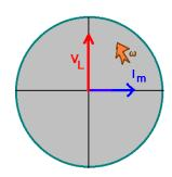
The current reaches its peak value 1/4 of a cycle later than the voltage reaches its peak value. For this reason, in this type of circuit obeying the initial assumptions it is said that the *current always* lags the voltage across an inductor by  $90^{\circ}$ .
