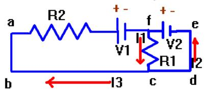
In a n-loop circuit, you will need to have n-1 current assignments.
