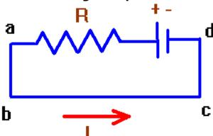
Here, a single loop has no junctions. Trace around the circuit after assigning a direction to the current:
