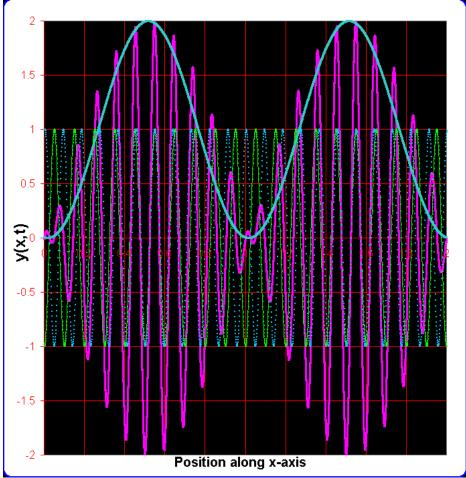
What I have plotted is a phase-shifted cosine curve (blue) which has a frequency of oscillation equal to the beat frequency  $f_b$ . Since it is the envelope of the beats that you would hear, this is indeed the beat frequency and not the "wrong" answer of 1/2 the beat frequency. Your ear would detect 2 beats in the picture shown above with the envelope correctly described with a beat frequency of  $f_b$ .
