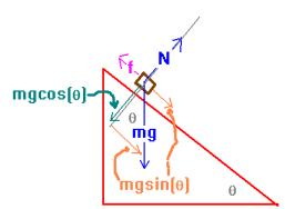
of friction between the inclined plane and the mass is  $\mu$ , at what angle should the plane be tilted in order for the block to slide with a constant velocity after being given an initial small push?
