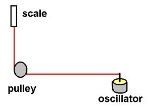
**Experiment 1.** Using the gram-spring scale connected to one end of the fat string and separate at least 1 meter distance between the oscillator and the pulley. You will need to measure the mass of your string and also the total length of it.
