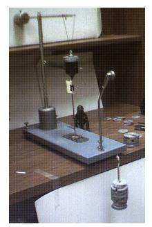
In today's lab, you will use the Welch Scientific Company's Centripetal Force Apparatus to verify the relationship between centripetal force, mass, velocity and radius. You may recall from class that for a mass moving in uniform circular motion, the centripetal force is given by:
