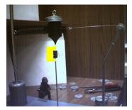
We could also vary the radius of orbit but this proves to be significantly more difficult so we will keep R fixed in this lab. The image to the left shows the apparatus.
