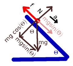
This shows the resolution of forces on an inclined plane. The gravitational force is reduced into parallel and perpendicular components to the surface of the plane. Doing this allows the acceleration to be parallel to the plane. We apply Newton's law here:
